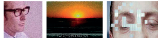
Examples for various video impairments: noise (left), video breakup (middle), block dropout (right)
